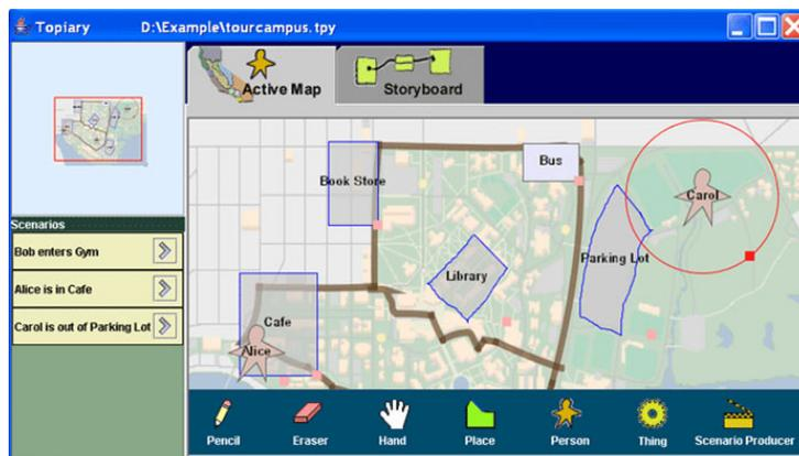
**Fig. 2.** A screenshot of *Topiary*, a prototyping tool for location-aware applications. Topiary uses Place Lab to allow the prototypes to use live location estimates
